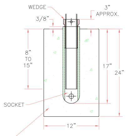
NON-REINFORCED CONCRETE FOOTING (SHALL BE USED UNLESS NOTED ELSEWHERE IN THE PLANS). FOUNDATION SHOULD TAKE APPROX. 1.6 CF OF CONCRETE. (APPORX. 17 POSTS CAN BE INSTALLED PER CUBIC YARD OF CONCRETE.)
